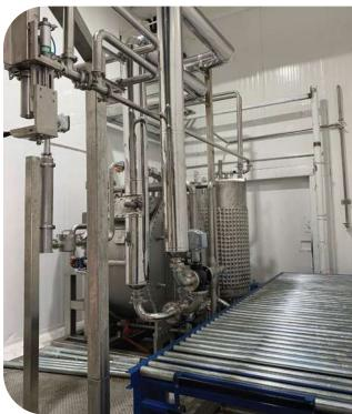
IceGen units are available in configurations with mass flow rates from 5 to 200 GPM and can deliver a daily output of 20 to 1,000 tons. Customizable actual system capacities are based on the weight of ice crystals fraction suspension in the solution and the type of freezing point depressant agents clients require. This process is flexible and can be automated to generate variable crystallization rates and sizes to meet different loads for distribution and ice suspension blending.
